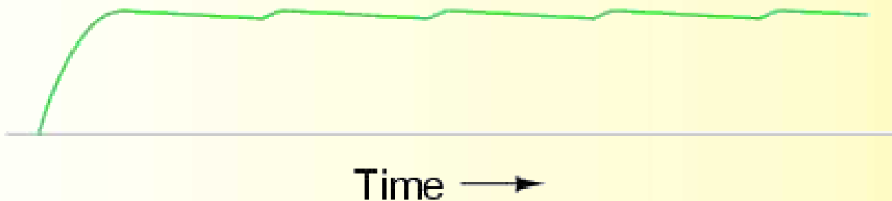
Full-wave, rectified DC voltage, with filtering
